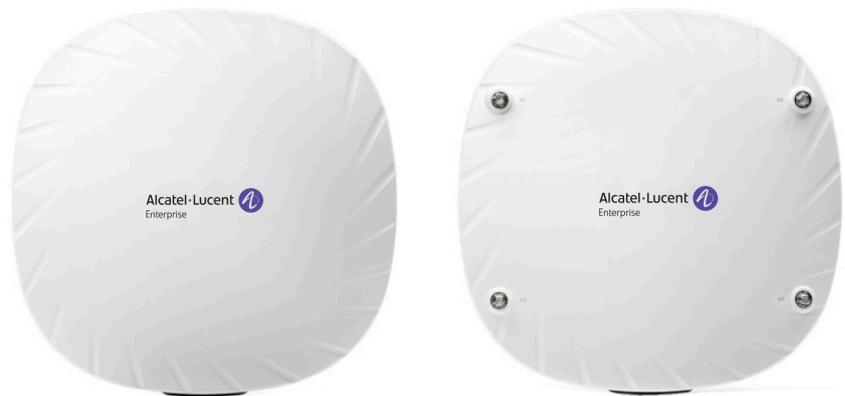
The OmniAccess 530 Series campus access points with 802.11ax technology are designed to deliver high performance access for mobile and IoT devices in environments where device density is high. The 530 Series uses 802.11ax features to simultaneously serve multiple clients and prioritize different types of traffic, which increases the data rates for both individual applications, devices and the overall network.
